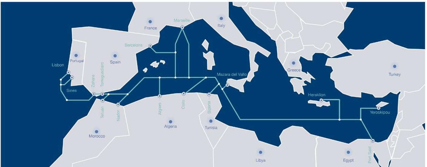
The construction has been awarded to industry leaders ASN and Elettra Tlc. The Medusa system is built on state-of-the-art 24-pair fiber optic Open Cable technology to meet increasing broadband requirements in the region, with 20Tb/s minimum capacity per fiber pair.
